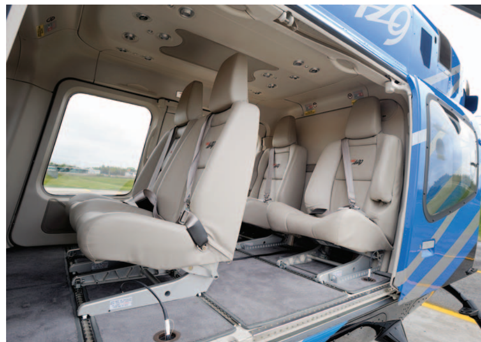
Versatility describes the 429's open cabin. Shown here are 18.5-in. seats in the front row and 21.5-in. seats in the back. Removing the back wall provides enough room for two stretchers and two attendants.
