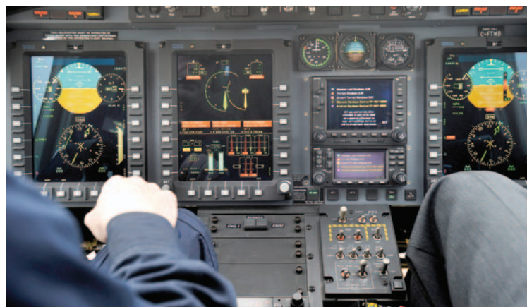
Bell test pilot Leo Meslin (left seat) describes the 429's cockpit to the author. Three large Rogerson Kratos displays, a Garmin 530 and a Garmin 430 dominate the instrument panel.
