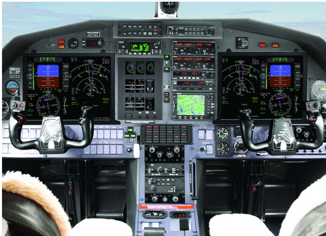
More cockpit retrofit systems in the category of this Pilatus PC-12 upgrade from Innovative Solutions & Support are entering service, putting pressure on manufacturers of the Part 23 avionics to provide top-level support. A push by some companies into the higher-echelon Part 25 realm will only add to the requirement to develop reliable components while keeping prices in check.
