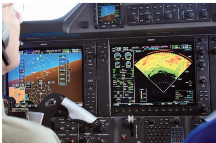
**The avionics suite in the Phenom 100 is the Prodigy, a version of Garmin's popular G1000. The system includes three interchangeable 12-inch LCD screens.**
