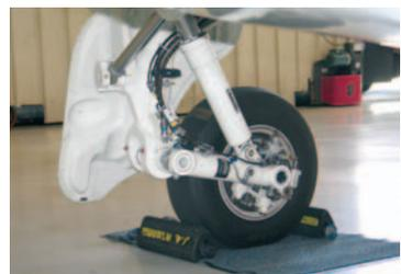
**The Phenom 100's trailing-link landing gear should help even new pilots deliver smooth landings.**
