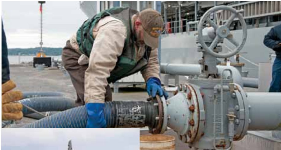
Above, a fuel distribution system operator secures a fueling hose during a biofuels transfer to the Military Sealift Command fleet replenishment oiler USNS Henry J. Kaiser. The oiler took on 900,000 gallons of a 50-50 blend of advanced biofuels before delivering the upload to machinery participating in the Great Green Fleet demonstration, to fuel aircraft such as the Hornet.
