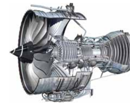
The improved Trent 1000, branded the Trent 1000-Ten, from Rolls-Royce will provide a modest but welcome one-percent increase in efficiency.
