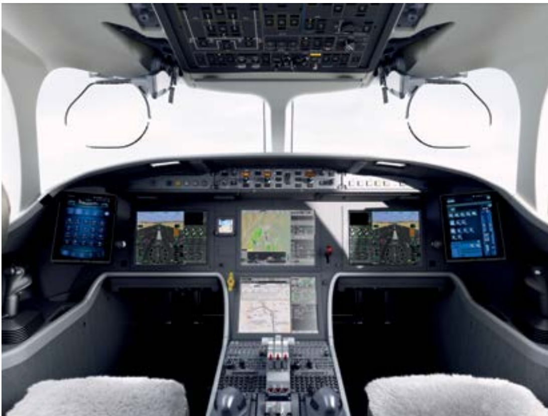
Sidestick-operated fly-by-wire flight controls make for a clean, uncluttered flight deck. The 8X's EASy III avionics system, based on Honeywell's Primus Epic suite, features synthetic vision and 3-D digital radar. The FalconEye HUD and combined vision system is optional.
