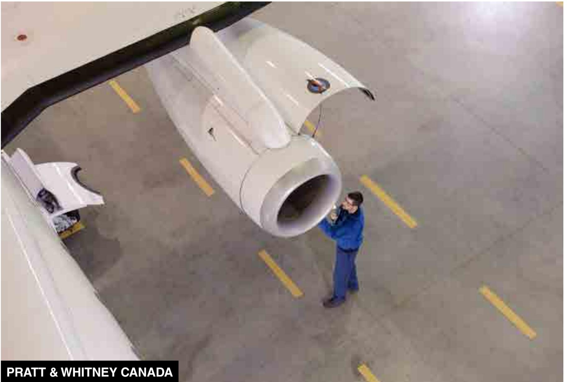
has begun the commercial introduction of an oil analysis program that “provides high visibility into the health and proficient operation of the engine without intrusive inspections. It detects tiny metal traces within engine oil enabling the identification of deterioration of specific oil-wetted components such as gears, bearings and seals. The technology is now calibrated for the G200 (PW306A), Phenom (PW617), Caravan (PT6A-114/114A), TBM (PT6A-64/66D) and PC-12 (PT6A-67B/67P).
