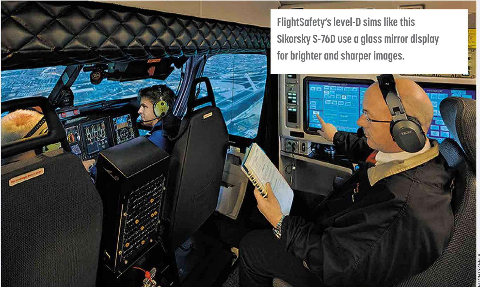
FlightSafety's level-D sims like this Sikorsky S-76D use a glass mirror display for brighter and sharper images.
