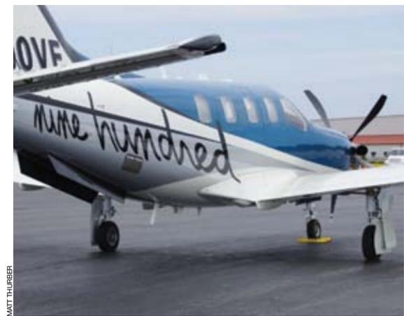
Sharp-eyed TBM fans will spot the smoother composite dorsal fin, new gear leg doors and winglets. The 900's five-blade Hartzell prop can be retrofitted to earlier TBMs.
