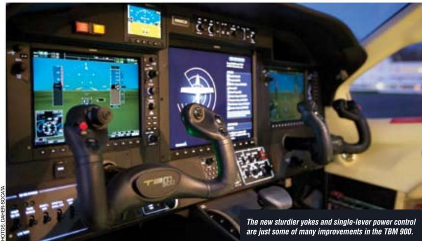
The new sturdier yokes and single-lever power control are just some of many improvements in the TBM 900.
