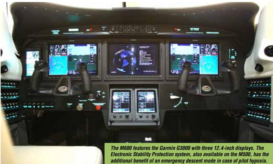
*The M600 features the Garmin G3000 with three 12.4-inch displays. The Electronic Stability Protection system, also available on the M500, has the additional benefit of an emergency descent mode in case of pilot hypoxia.*
