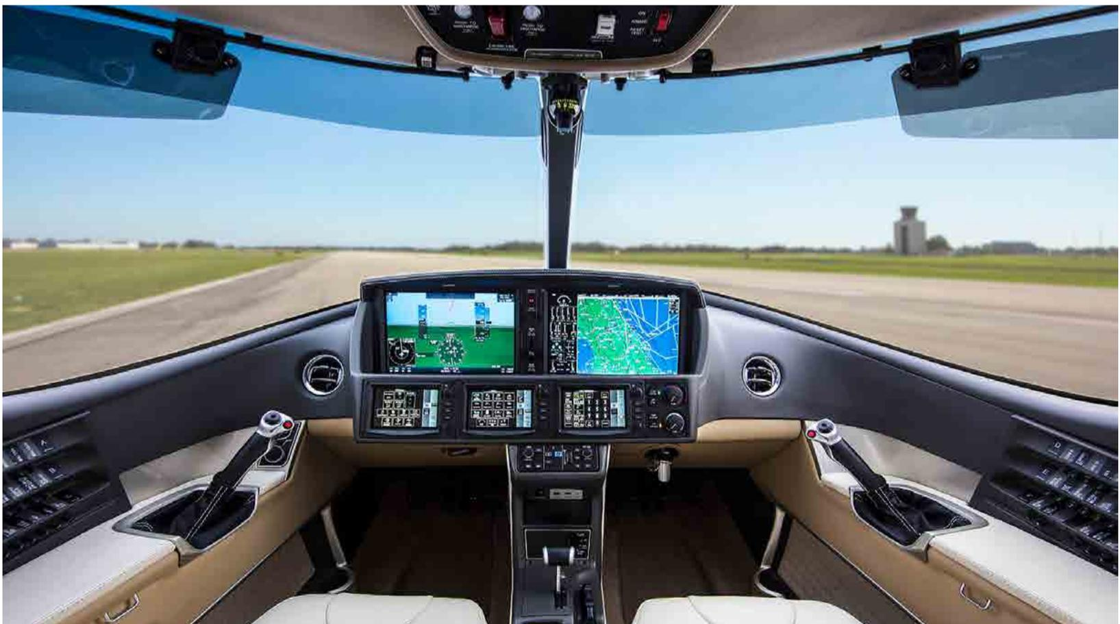
**The Garmin-based cockpit of the Vision Jet will feel familiar to pilots of the SR22. In the jet, however, the Perspective Touch employs G3000-based touchscreen controllers.**
