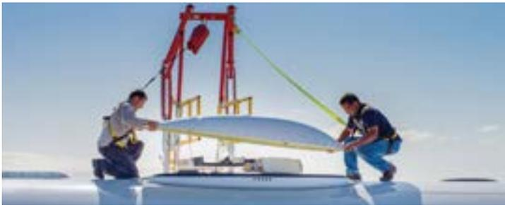
Technicians install the antenna for a JetWave system on an airliner fuselage.
